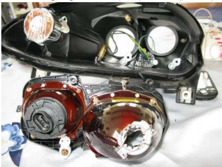
14. Remove these 3 screws from the dipped beam assembly (photo 13).
