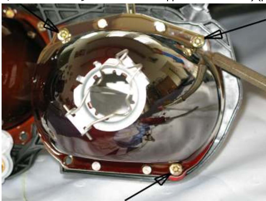
14. Remove these 3 screws from the dipped beam assembly (photo 13).
