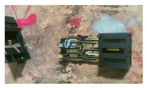
5) The resistor is on the V+ (12v) the 2 leds have 1 leg common up this V- GROUND
