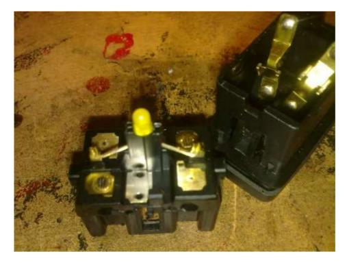
Note left leg of the LED is the positive side V+
