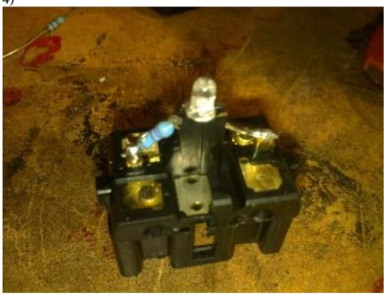
Solder the resistor in place if required (1k is less bright than 750 ohms) I use 820 ohms
