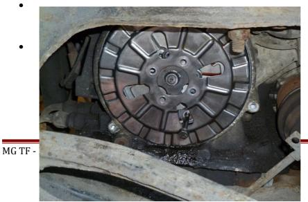
Remove and discard the 4 X 8mm bolts securing the pitot chamber Rotate the pitot chamber sufficiently to gain access to the lower right hand oil pump bolt which secures the short pitot tube. Remove the bolt and using
