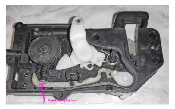
As I had already removed the Super Locking Mechanism, I then restricted the movement of the Main arm by drilling a small hole and screwing in a Screw. There needs to be a slight gap between the Arm and the Screw so that one of the Switches is properly engaged. Now the Main Arm has only 2 positions, Lock and Unlock.
