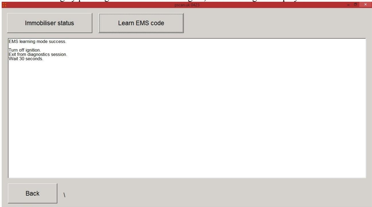
The synchronization of the EMS code between the engine control unit and the Lucas 5AS alarm unit has been completed. The vehicle must be able to start.
