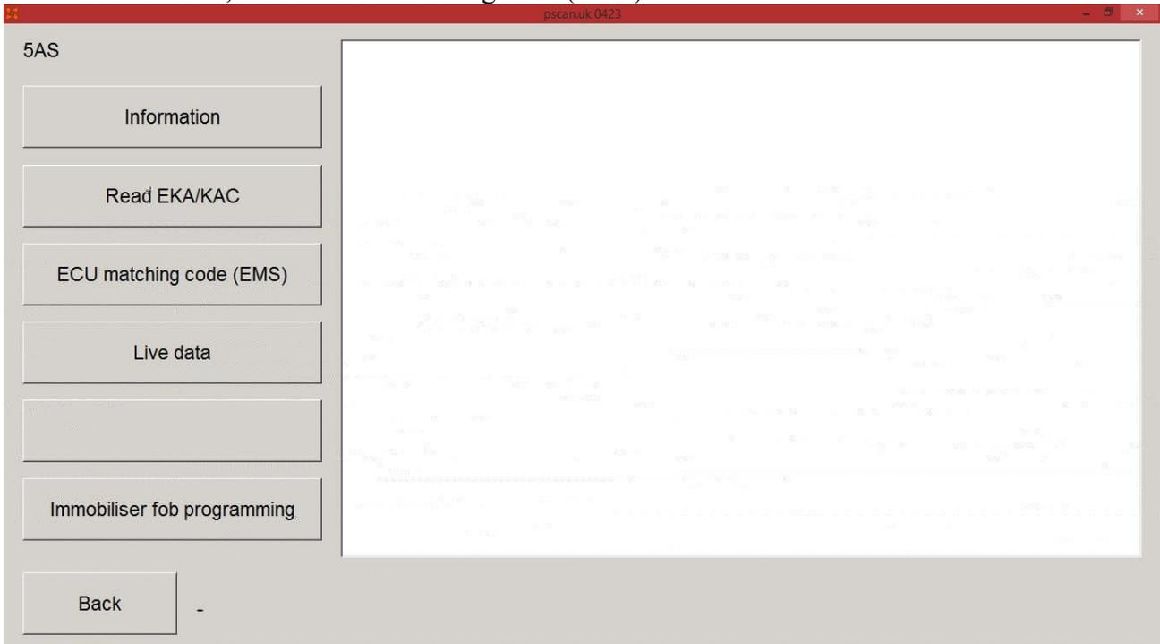
Read EMS code "Read EMS". It is possible to modify this code with the case "Increase digit 1" and "Next digit". Validate on "Write EMS" then return to the main page.
